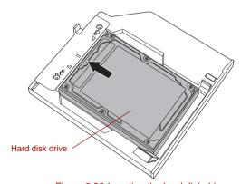
Figure 3-23 Inserting the hard disk drive
